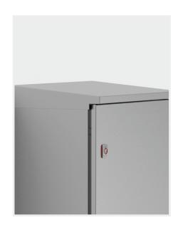
**Description:** To be fitted as an outdoor shelter on stainless steel wall mounted enclosures. The roof is slightly sloped and has a drip strip. Machining is required. Dimensions of the enclosure will be increased by H: 60 mm, W: 20 mm and D: 20 mm.
