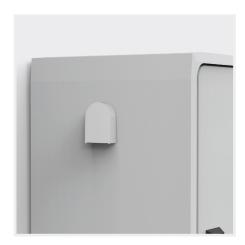
**Description:** Two air vents must be mounted per enclosure to ensure sufficient air circulation and prevent water condensation. Air vents are preferably mounted in the upper and lower part of the enclosure. Degree protection: IP 44.
