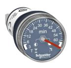
Harmony XB5, Panel mounted timer monofunction, plastic, Ø22, time delay 3...60 min, 24 V DC
