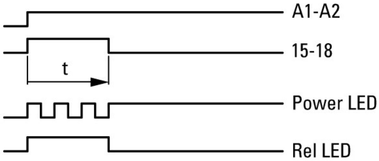
21 Fleeting contact on energization
